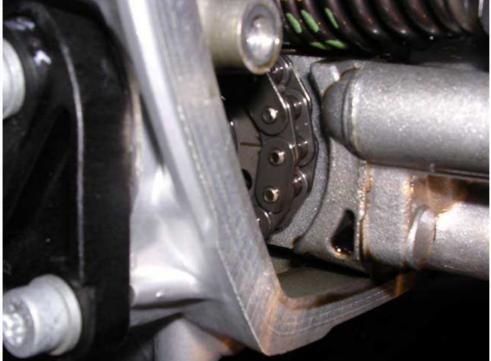
The right side of the 12GS has a cam arrow like on the R11 series, and it worked the same way. Have the arrow point straight out, and check the valves to make sure both intake and exhaust are loose. If not, rotate the engine so the arrow comes around again.
