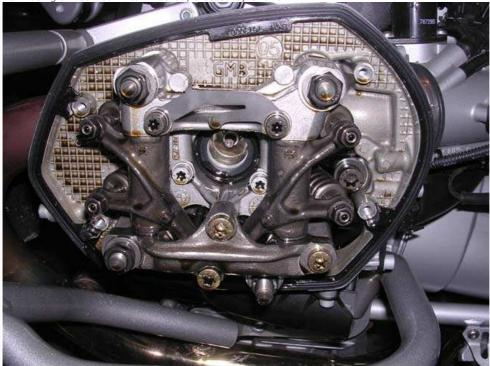
The cover came off the same as the 11GS, and easily cleared the H&B crash bars. However, the front engine cover would not even come close to coming off with the crash bars, so I pulled the plugs and rotated the engine using the rear wheel with the trans in 6th gear.
