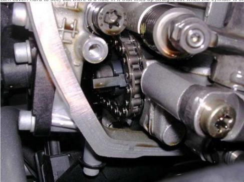
If you look back over on the right side, this is what you see when the left is at TDC, if the valves aren't loose to the touch, rotate the engine so the cam rotates 360 degrees.
