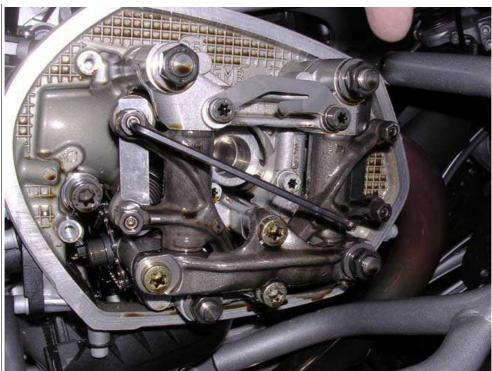
Tighten the lock nut without disturbing the position of the allen wrench. I hold it in place and tighten the locking nut. Pull from the center, and if the resistance is even, you have the adjusted correctly. There should be some slight resistance, but it should be easy to move the feeler gages. Rotate the engine and do the other side.
