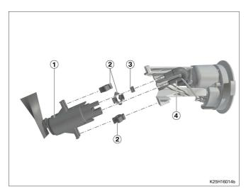
(4), making sure that the gasket is correctly seated.
